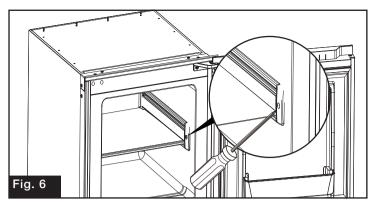
4. Repeat steps 2 and 3 to loosen the shelf fixing screw on the other side. Pull to remove the shelf out from its original position. (Fig. 7)
