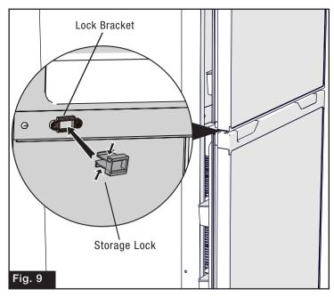
3. Close the doors so that the door latch engages with the storage lock.
